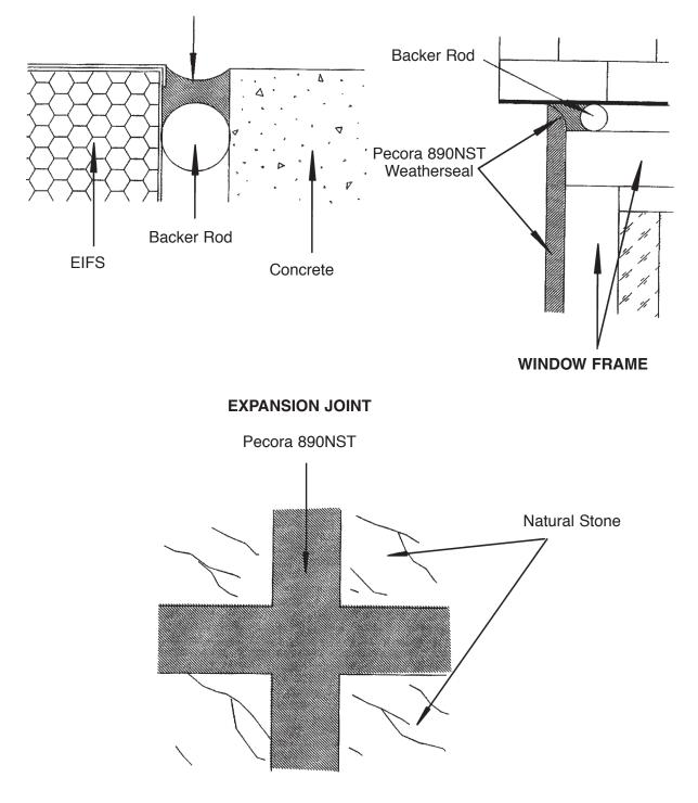
Sealant should be applied in a continuous operation using sufficient pressure to fill the joint and make complete contact to the joint sides. Tool the sealant slightly concave using solvent or dry-tooling techniques. Contact Technical Services prior to tooling with solvent. Do not tool with soap or detergent and water solutions.
