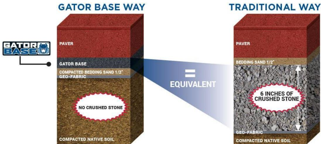
When laying different thickness of pavers or stones, adding a second layer 1/2" (13 mm) of loose bedding sand on top of the Gator Base™ is also an accepted method of installation.
