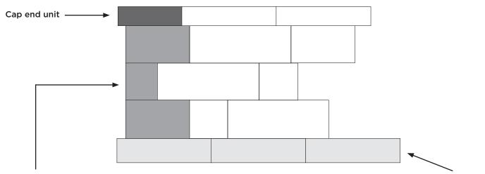
This shaded area represents wall end units. Every other wall end unit is cut in half. Torpedo<sup>™</sup> base course
