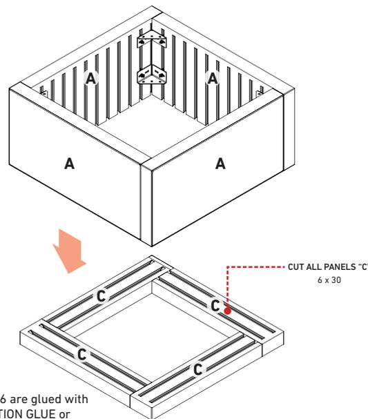
**NOTE:** The panels 18 x 36 are glued with 6 x 36 using CONSTRUCTION GLUE or STRUCTURE BOND
