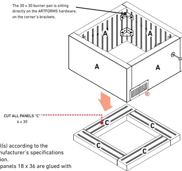
Ⓞ Cut panel(s) according to the burner manufacturer's specifications for ventilation.
