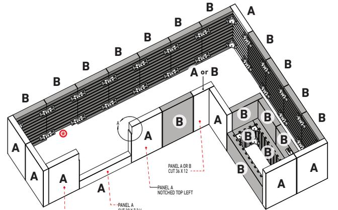
⊕ Cut panel(s) according to the BBQ manufacturer's specifications for ventilation.
