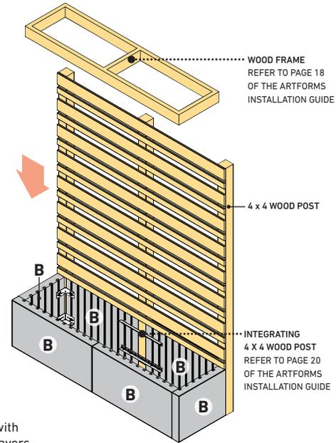
**NOTE:** Panels "B" can be replaced with panels "A" to equilibrate the pairs/layers.
