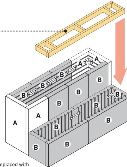
**NOTE:** Panels "B" can be replaced with panels "A" to equilibrate the pairs/layers. Panels "A" can't be replaced by the panels "B".
