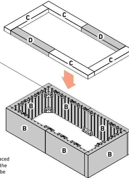
**NOTE:** Panels "B" can be replaced with panels "A" to equilibrate the pairs/layers. Panels "A" can't be replaced by the panels "B".
