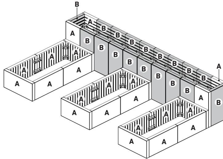
**NOTE:** Panels "B" can be replaced with panels "A" to equilibrate the pairs/layers. Panels "A" can't be replaced by the panels "B".
