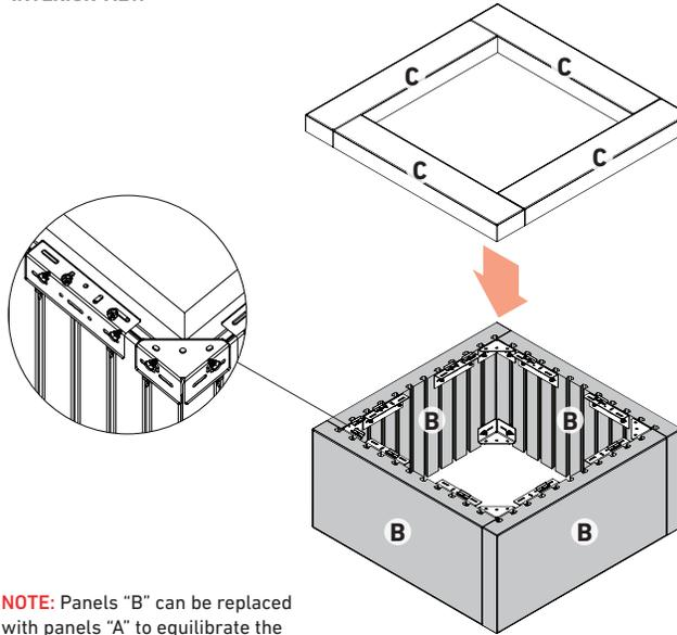
**NOTE:** Panels "B" can be replaced with panels "A" to equilibrate the pairs/layers. Panels "A" can't be replaced by the panels "B".
