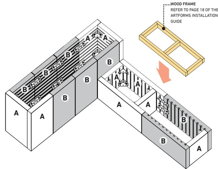
**NOTE:** Panels "B" can be replaced with panels "A" to equilibrate the pairs/layers. Panels "A" can't be replaced by the panels "B".
