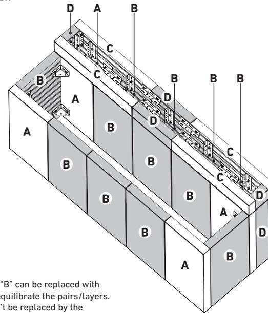
**NOTE:** Panels "B" can be replaced with panels "A" to equilibrate the pairs/layers. Panels "A" can't be replaced by the panels "B".
