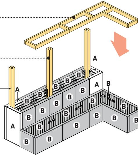
**NOTE:** Panels "B" can be replaced with panels "A" to equilibrate the pairs/layers. Panels "A" can't be replaced by the panels "B".
