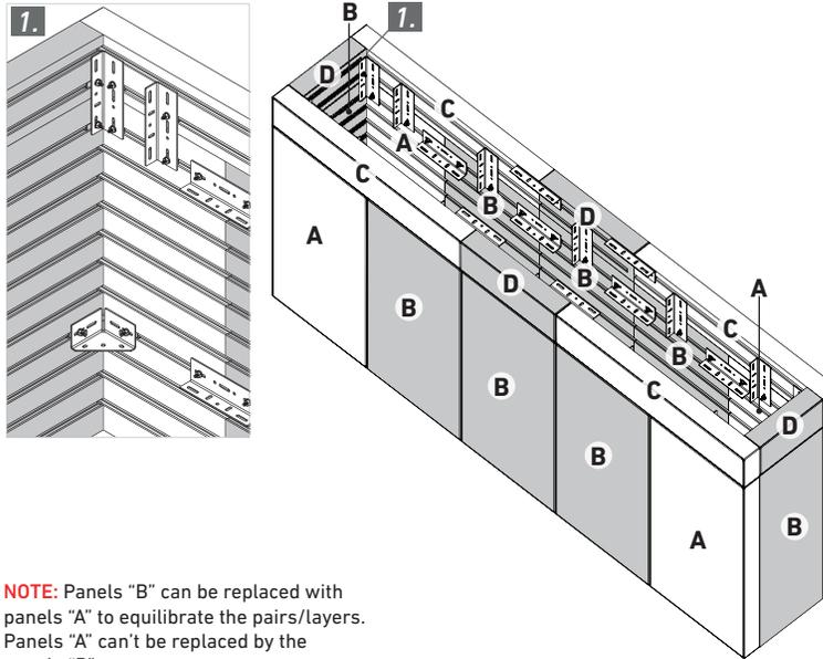
**NOTE:** Panels "B" can be replaced with panels "A" to equilibrate the pairs/layers. Panels "A" can't be replaced by the panels "B".
